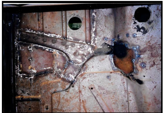
ANDREW REPAIRING UNDERSIDE OF FLOOR, LOTS OF CLEANING, GRINDING & WELDING
