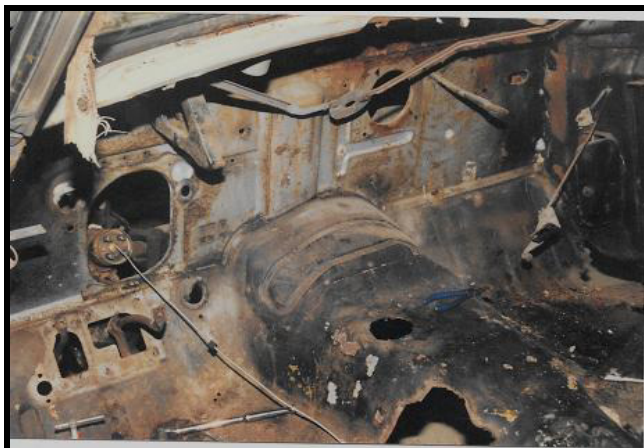
MANY AREAS OF THE BODY HAD TO BE STRENGTHENED BEFORE TAKING IT OFF THE FRAME
