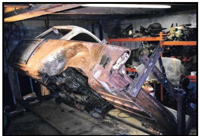
BODY COMES OFF FRAME AND MOUNTED TO ROTISSERIE
