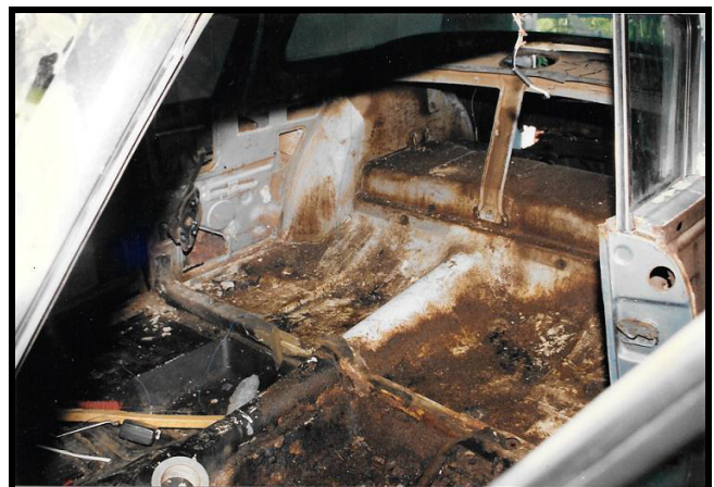
MANY AREAS OF THE BODY HAD TO BE STRENGTHENED BEFORE TAKING IT OFF THE FRAME
