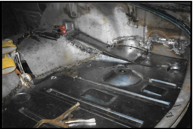
NEW TRUNK FLOOR INSTALLED
