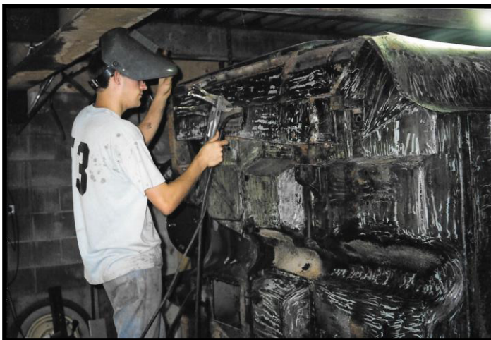
ANDREW REPAIRING UNDERSIDE OF FLOOR, LOTS OF CLEANING, GRINDING & WELDING
