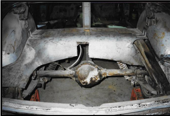
ORIGINAL TRUNK FLOOR REMOVED
