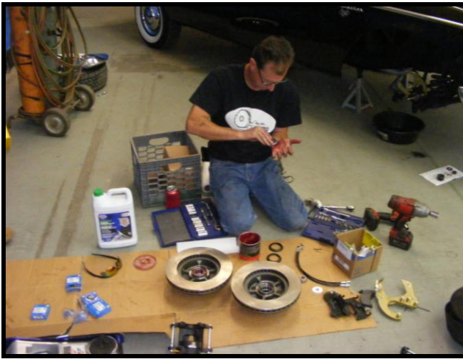
NEW PARTS READY TO INSTALL. MIKE PACKING THE BEARINGS WITH GREASE
