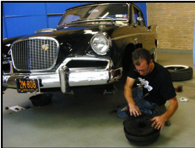
MIKE MYERS SHOWING HOW TO DO A DISC BRAKE CONVERSION ON BOB STOWELL'S '57 SILVER HAWK.
