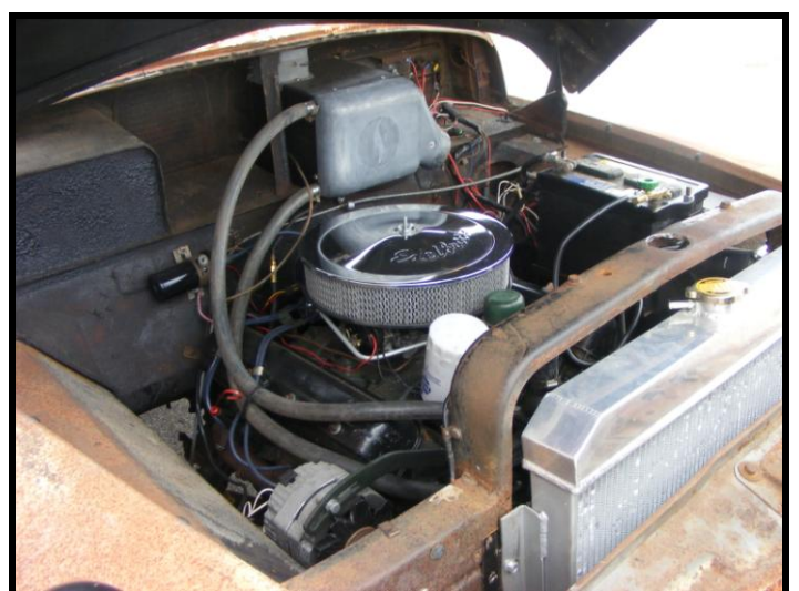
CHRIS REPLACED THE ORIGINAL 6 WITH A 259 V8
