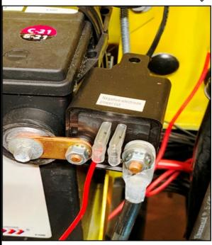
Installation on the negative battery post was really straight forward with simple hand tools. Connecting the red wire to the positive battery post completed the job; all in less than 15 minutes start to finish. Now I can disconnect the battery with a simple push button and the car cannot be started without the remote.
