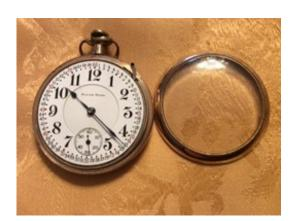
This is a South Bend model 227, size 16 railroad grade and approved watch, note the lever above the "2". The face/crystal had to be removed and the lever extended in order to change or adjust the
